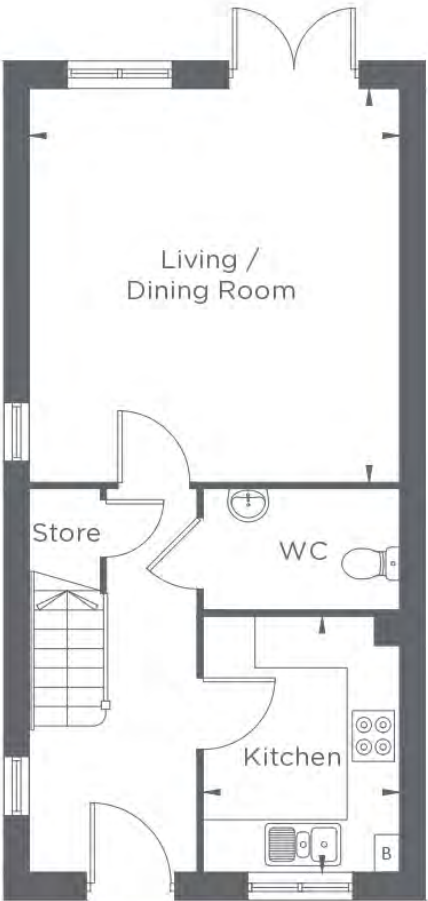
GROUND FLOOR *B = Boiler
