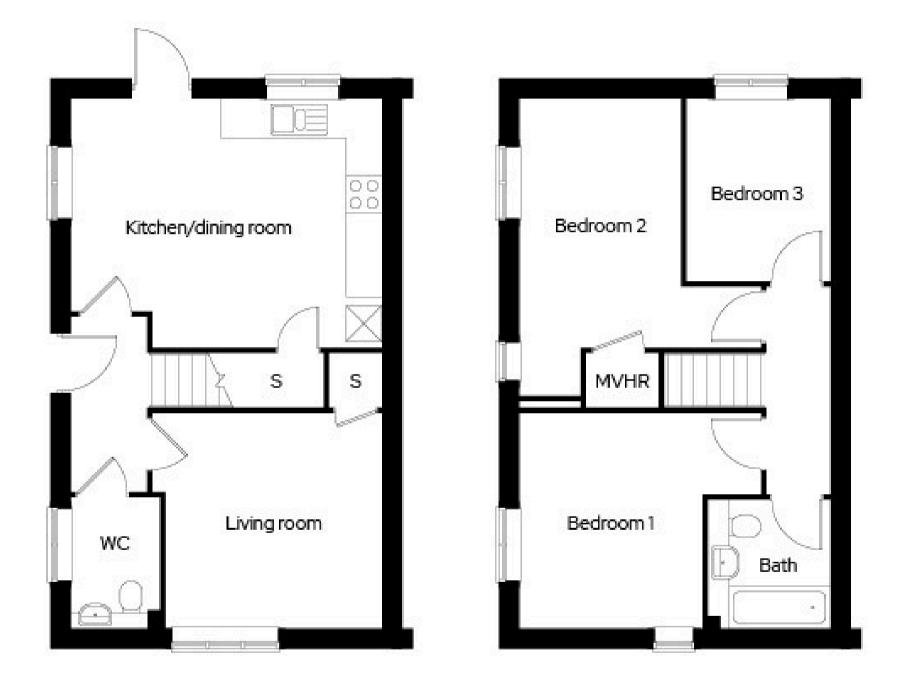
\* Mirrored plot MVHR Mechanical ventilation & heat recovery S Storage
